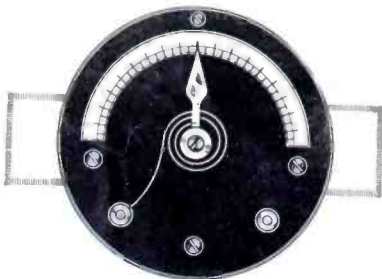
Be Certain of Proper Connection in Variables. A Little Hair Spiral Spring Does the Stunt.
